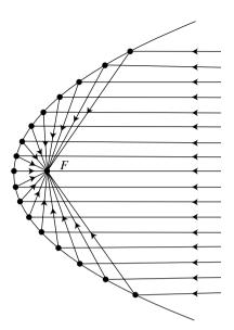
Fig. 10.2. Reflective property for a parabola
