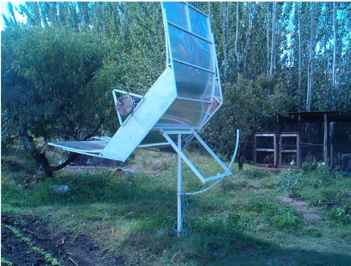
Fig. 2: View of device from rear, and illustrating dual axis tracking and adjustment.
