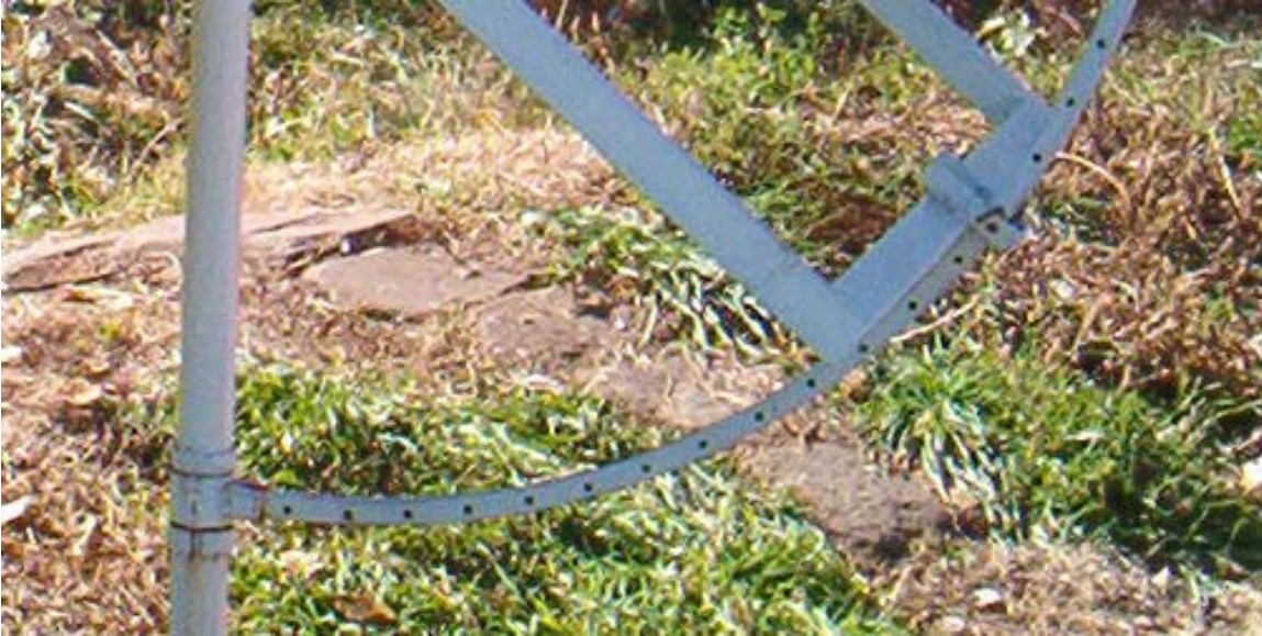
Fig. 11: Detail of altitude adjustment; note that radius arm is able to swivel on the vertical support. Device is locked in place with a pin.
