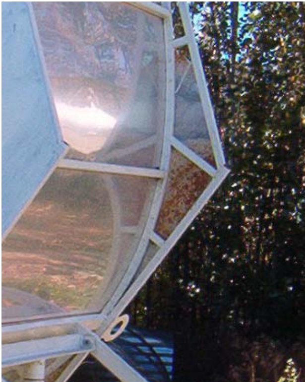
Fig. 10: Truss section used to maintain parabolic Profile. Note circular aiming device on far edge.
