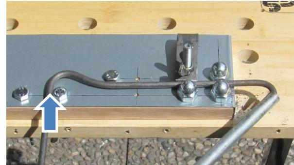
Prepare the forth bend, positioning the workpiece with its left part at the right bolt head and fixing with the wing nut.
