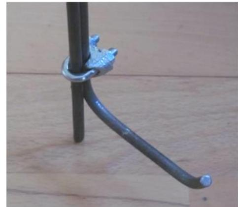
Rope clamps may provide an alternative for connection of the tripod legs if welding equipment is not available.
