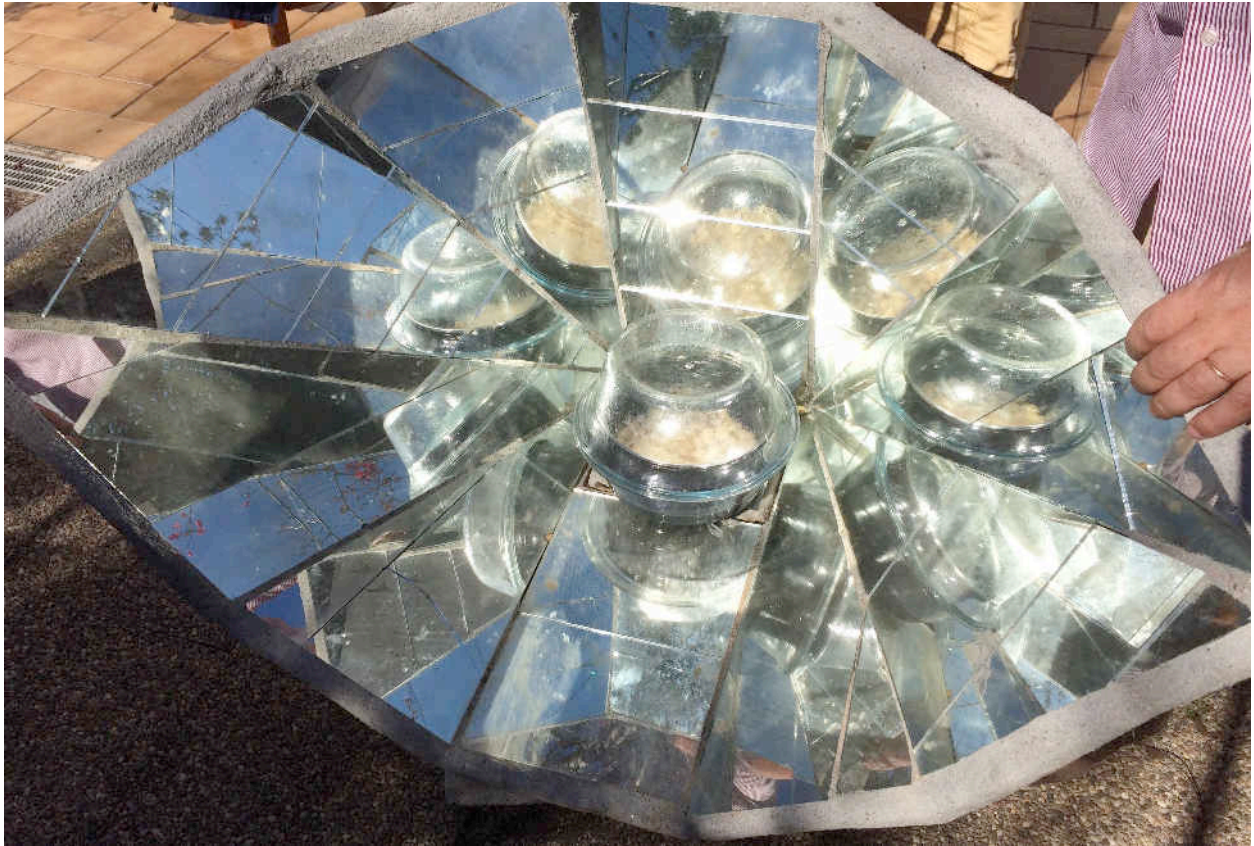
Photo 2: A funnel cooker made of concrete by Celestino Ruivo, Portugal, It can be left outside throughout the year. A weight of 80 kg protects these models from theft.
